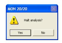
3. Click **Yes** and the analysis will stop at the end of the current cycle. Use the *Mode* column on the **GC Status Bar** to monitor the status of the operation. When the analysis has halted, the Mode value will be "Idle".
